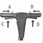
8. Push the both safety button "A" and "B" entad, and then tighten the switch that both left and right on the lever "C" and "D", to running the motor
